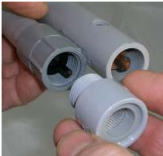
3. Screw in screen fitting hand tight.
